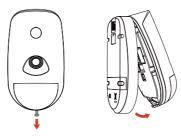
Step 4. Install the detector.
