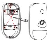
(2) Complete wiring terminal's wiring and fix the rear cover to the wall with 4 screws(PA $_3.5 \times 25$ ). Install the front cover.
